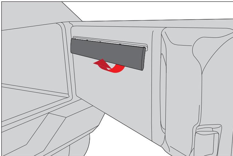
3. From the top edge, insert plastic hooks on plastic trim through top row of cut outs in Tailgate Cover.
