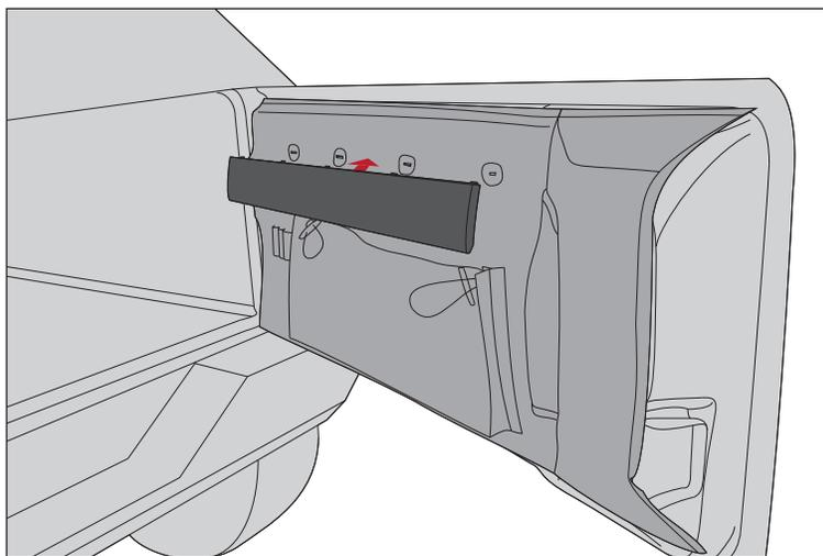
5. Remove adhesive backing from tape. Pull edges of Tailgate Cover tightly over tailgate and press firmly to adhere to tailgate.
