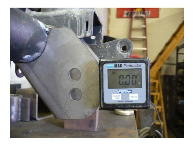
6. Position the passenger side bracket opposite. The easiest way is to measure from the machined edge adjacent to the weld on the inner C. Measure the driver side then make the passenger side bracket the same dimension. The dimension should be close to 5 ½ to the outside edge of the new lower control arm bracket. Tack weld into place.
