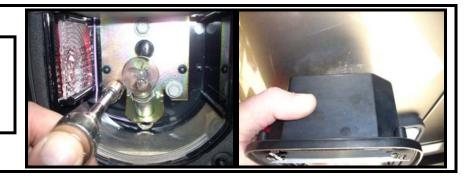
**Step 5:** Carefully pull the tail light wiring through the hole. Guide the connector through the hole.
