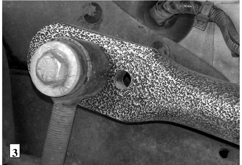
1. Entirely remove the front factory sway bar and end links. Keep the hardware as some of it will be reused in the installation.
