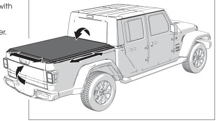
NOTE: When opening the cover, be sure to stow the tail clamps into the cover bow to prevent damage to the tarp when folded.
