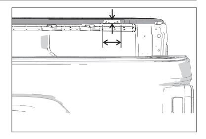
3. Front/ Cab Brackets, insert the cab bracket screw (1) through the cab bracket washer (2) then through the upper hole of the cab bracket (3). Slide a second washer (2) on the screw on the backside of the bracket and thread into the well nut (4).
