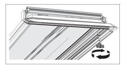
6. Place the cover onto the truck bulkhead and bed rails, making sure to slide the cab clamp threaded rods (2) through the cab clamp brackets (3). Align both sides.
