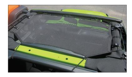
Before installing flip soft top to Sunrider feature or lower top to full down position. Freedom panels will need to be removed for installation on hard top vehicles. Slide front side Velcro straps through windshield footman loops and secure (fig.1). Loop rear Bungee straps over factory sports bar and back to strap button (fig.2)
