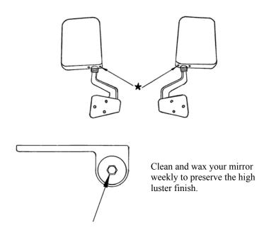
Note: If mirror will not pivot, for adjusting loosen nut at the bottom. Make sure nut is tightened otherwise mirror will vibrate.
