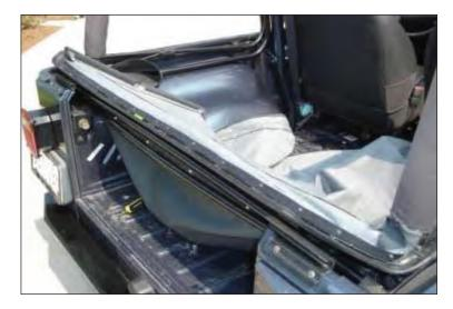
7. Lay new soft top fabric in rear of vehicle with bottom side up. Ensure plastic strip on fabric is facing up and aligned with front edge of windshield header. Locate round hole that marks center of plastic strip and install first screw to ensure fabric is centered on header. Install remaining screws removed in step 6.
