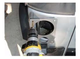
6. Cut out the rear of the JK tub to allow for clearance for the 4" LED tail light. This is a trial and error fit. Photo on the right is the finished result.
