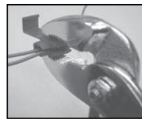
Crimp clamp with pliers, then close lock.
