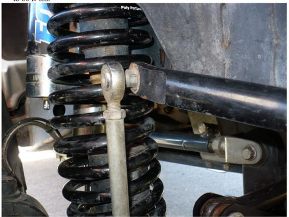
Attach the disconnect pins to the frame brackets using a flat washer on both sides and nylock nut as shown below. Slide the pins to the middle of the slotted hole. Tighten the nut to 40 ft-lbs.
