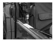
**Step 4:** Take a mounting bracket and place it in position on the tub centered around the mark you made in Step 3. Then mark the holes making sure that they are centered on the top lip of the tub.
