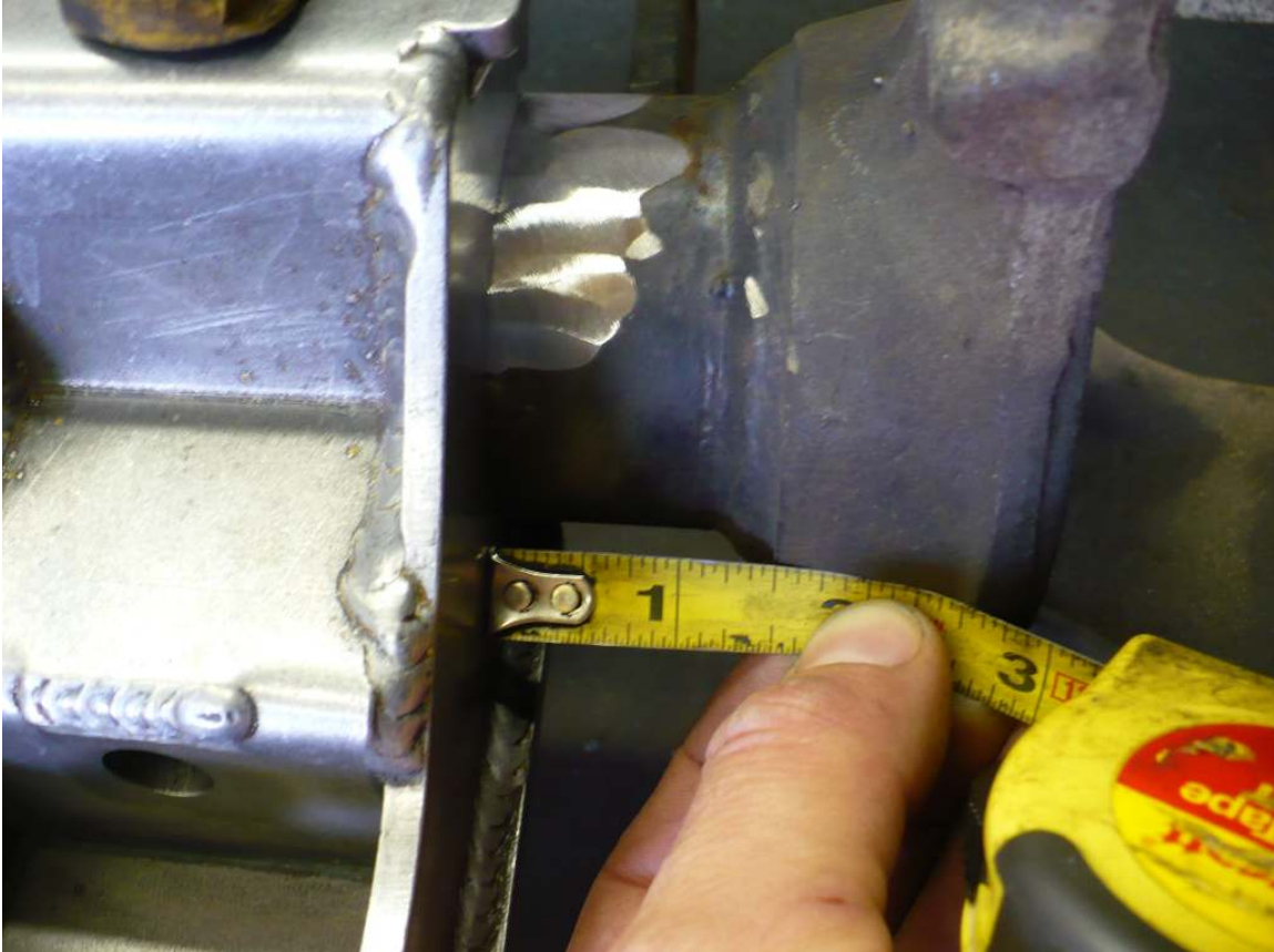
b) The outer edge of the lower shock bracket should be about 1 ½” from the machined edge adjacent to the weld on the inner C.
