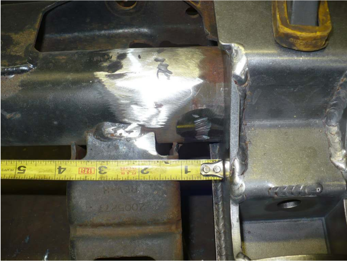
b) The outer edge of the lower shock bracket should be about 1 ½” from the machined edge adjacent to the weld on the inner C.
