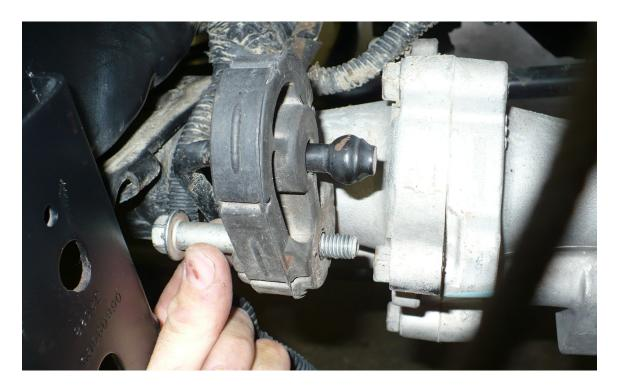
3. Loosen the front stabilizer bar retainer bolt on the passenger side to lower the stabilizer bar enough to rotate the disconnecting stabilizer bar unit up and in front of the radiator. You will need to notch the lower radiator plastic cover to clear the electrical plug.
