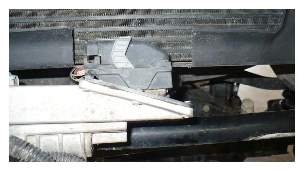
4. Tighten the front stabilizer bar retainer bolt. To 45 ft-lbs.
