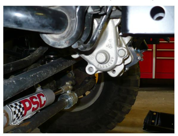
2. Remove the disconnecting stabilizer bar tension link bolt.
