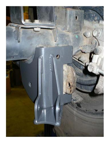
8) Align the bracket so the 4.5" long 9/16" bolt provided in the kit can be slid through. Put a washer on both ends and start the stover nut. Do not install the control arm at this time. Do not fully tighten at this time.
