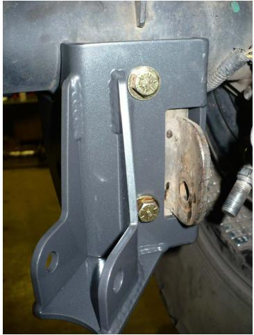
(NOTE: If bracket is welded on, now is the time to do so. Clean areas where planning to weld and weld bracket on at this time. See picture below for weld area recommendations.
