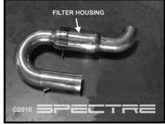
Insert air filter into the short intake tube (with the filter housing) until the lip of the filter is in contact with the edge of the tube. Install the collar clamp boot halfway over the filter housing and position the collar clamp over the boot. Insert the long tube into the boot, positioning it as shown. Snug up the clamp, but do not fully tighten as you will need to rotate the tubes to position them in a future step.
