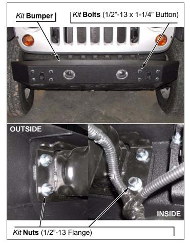
4. Note: 2010 & 2011 Models mark and drill passenger side lower crash bar. Mark and drill (using a 1/2" drill bit) passenger side lower crash bar so *kit* Bolts (1/2-13x1 1/4 botton head) may sit flush through bumper.
