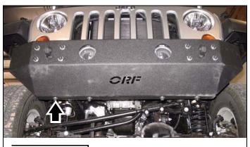
Drill 1/2" hole on Passenger side crash bar.
