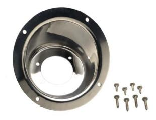
Remove the gas cap and the plastic holding strap. Remove the eight screws holding the existing filler neck. Install the new Stainless Steel gas filler neck using the stainless screws provided. The four 3/4" Lg. Screws go on the outside and the long screws go on the inside.
