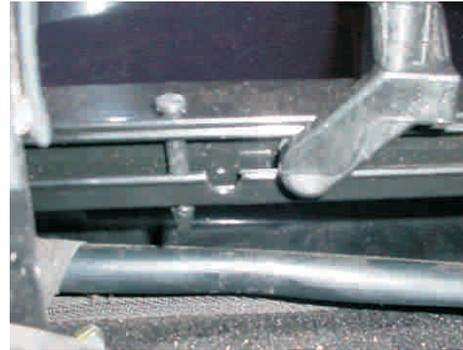
4. Unfold Passenger Upper Side Rail towards the front of the vehicle until it reaches the Passenger Upright Pin. Insert the plastic Upright's Pin through the Side Rail's hole and lock it in place by sliding the square clip to the opposite side. **NOTE:** Make sure the Upper Side Rail is properly secure prior to installing the soft top. Damage to the vehicle or personal injury can occur if not installed properly. Repeat this step for opposite side.
