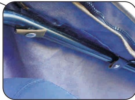
3. Insert the front of the top into the Windshield Channel.
