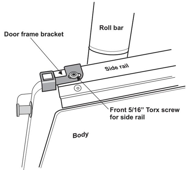
NOTE: for Cj7 additional holes must be drilled in the mounts and sheetmetal screws must be used to attach to the windshield frame. Screws not provided. (See above)
