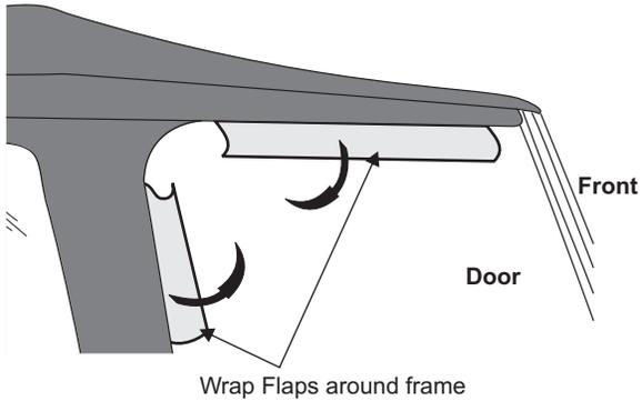
15. Wrap the door flaps around the door surrounds and attach back on the inside of the top with the velcro. Repeat for other side.
