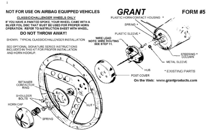
1. Point wheels straight ahead and disconnect battery or pull horn fuse before starting removal of the old wheel so horn won't short out and blow during installation.
