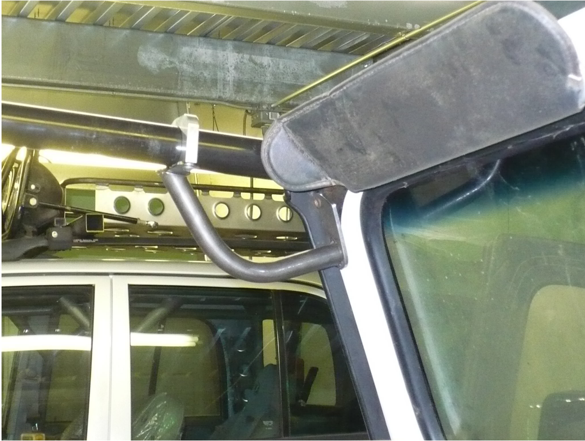
Fully installed YJ raw steel handle.
