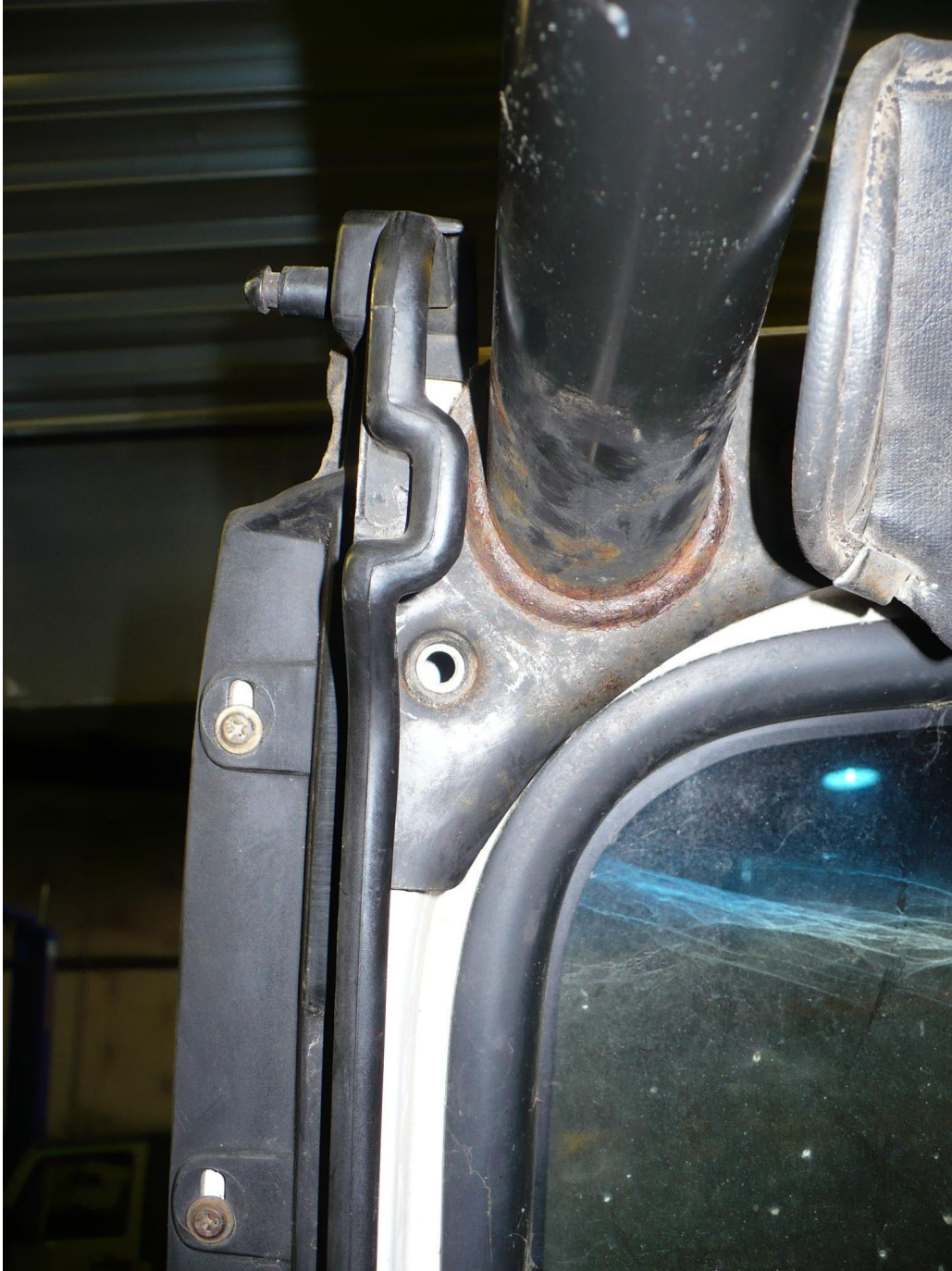
Outer Torx head bolt removed.
