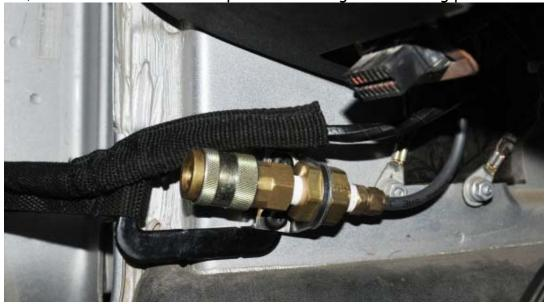
22. If using a front bumper air coupler, the following is a cleaver protected and hidden location:
