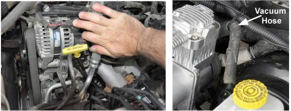
4. Loosely zip tie the vacuum hose as indicated in the previous picture, in order to assure at least  $\frac{1}{2}$ " clearance around the compressor head.
