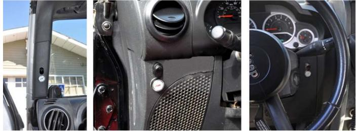
10. 3/8" Black Hose and  $\frac{1}{4}$ " FPT X 3/8" Barbed Fitting (Hose and Fitting supplied with compressor) – Rout the air intake hose as indicated in the following two pictures:
