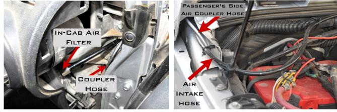
11. Air Couplers, Brass Compression Fittings, Air Coupler Brackets and Long Hoses – Using a Torx Wrench, install the In-Cab Air Coupler/s according the following picture:
