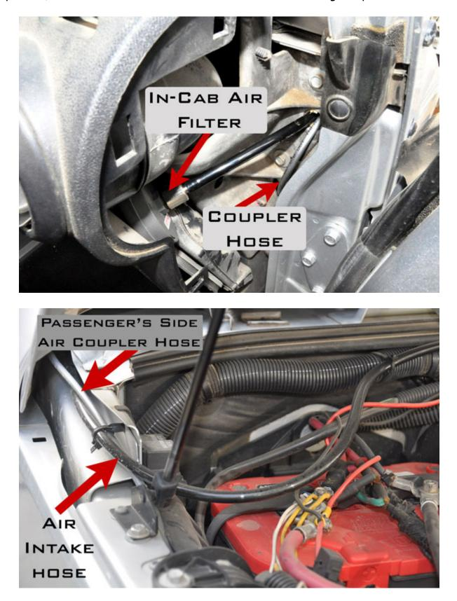
21. Air Couplers, Brass Compression Fittings, Air Coupler Brackets and Long Hoses - Using a Torx Wrench, install the In-Cab Air Coupler/s according the following picture:
