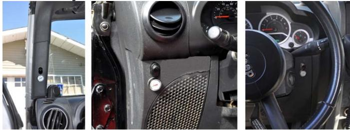
20. 3/8" Black Hose and  $\frac{1}{4}$ " FPT X 3/8" Barbed Fitting (Hose and Fitting supplied with compressor) – Rout the air intake hose as indicated in the following two pictures:
