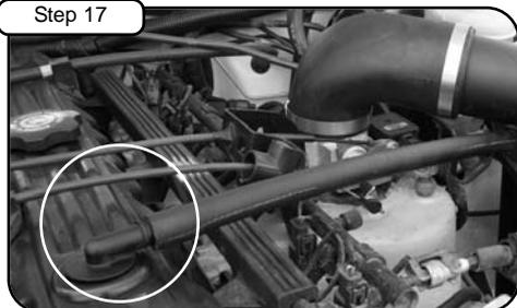
Attach 1/2" hose to crankcase engine side.
