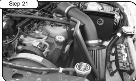
Install trim seal on housing. Your installation is now complete. Make sure you tighten all clamps and check all electrical connections periodically. Thank you for choosing aFe!
