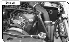
Install trim seal on housing. Your installation is now complete. Make sure you tighten all clamps and check all electrical connections periodically. Thank you for choosing aFel
