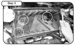
Loosen the 2 bolts and 1 nut holding in bottom half of air box using 12mm socket or wrench. Save all hardware for later use (see step 9).
