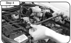
Remove crankcase line from valve cover.
