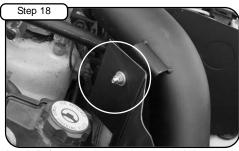
Install flat/wavy washers and nut to isolation mount. Tighten both sides with 10mm socket or wrench.
