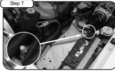
Loosen nut holding in ECU bracket with 12mm socket or wrench and remove. Save for later use (see step 10).
