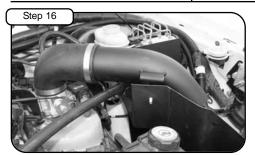
Insert tube in coupler. Place isolation mount in hole of housing.
