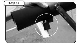
Install isolation mount to bracket with flat/wavy washers and nut provided. *Do not tighten.*
