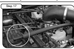
Attach 1/2" hose to crankcase engine side.
