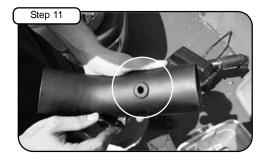
Install grommet in new intake tube.
