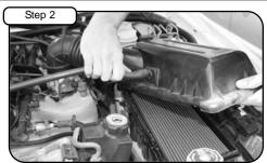
Unclip upper half of air box and pull back crankcase line.
