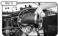
Install reducer elbow coupler to Throttle Body with clamps provided. *Do not tighten.*
