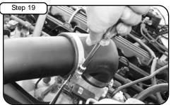
Tighten all clamps using 5/16" nut driver.
