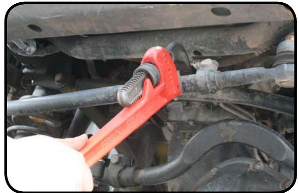
27. Re-torque all fasteners after 300 miles.
