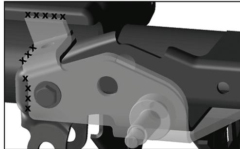
**HINT:** Be sure to include area on factory coil spring bracket and lower base of Relocation Bracket where it terminates just before it makes contact with axle tube.
