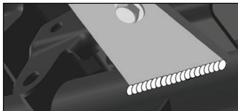
**IMPORTANT:** Avoid overheating axle tube and factory track bar bracket by welding a small section and allowing the surface to cool off regularly.
