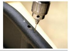
Route the wiring harness through the fender flare using a wire to help guide the harness through. Route the wire down through the drilled hole the and out the access hole.
