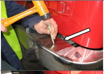
1. **ALL MODELS.** Locate laser cut circles on RH side of bar. Punch out using a centre punch. Clean any burrs and paint holes.
