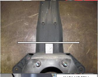
20. **JK.** Mark a line across the JK wheel mount as shown where the square access hole stops. Using a cutting disc or similar remove stop light section from mount. De-burr and paint surfaces.
