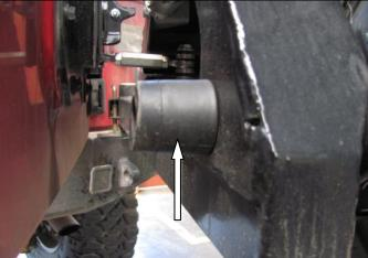
10. **JK.** Pull out the two rubber tyre rests from the JK tailgate and cut to a length of 50mm. Fit to holes provided in carrier.
