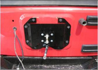
8. Install bracket to vehicle and tighten all bolts.
