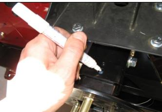
25. Move wheel mount inwards 10mm. This will place some load on the tyre when all is secured. Mark hole position, drill to 10mm and secure using M10 SEMS bolt and M10 flange nut.
