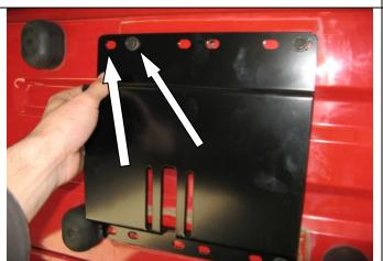
3. **FOR YJ-TJ.** Remove O.E tailgate bracket and stop light if fitted. Remove lower left bump stop from tailgate and plug hole using M6 bolt and flat washer. When bolting tailgate bracket to vehicle remember TJ uses holes to the left, YJ uses holes to the right. Secure using original hardware. Retain bump stop for fitment to arm.
