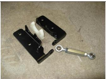
4. **ALL MODELS.** Lay out arm stop bracket and components as shown. Fit M10 left and right thread nuts to rod ends before fitting to turnbuckle. Secure nylon block to brackets using two M6 x 30mm bolts, flat washers and M6 nyloc nuts. Secure rod end to brackets using M10 x 35 bolt, Spring washer, flat washer and flange nut.
