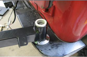
14. ALL MODELS. Place bottom plastic bush in arm (tapered version) and place arm onto spindle. It may need a tap with a soft hammer. Place top bush (square shoulder) into arm by tapping with a soft hammer. Secure using M20 nyloc nut and flat washer. Tighten so slack is taken up.
