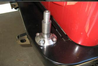
2. Place long shaft in centre M20 hole. Fit support hub over main shaft and line up the three M10 mounting points with holes in bar as shown in photo. Support may need to be tapped on using a soft hammer. Secure using M10 socket head cap screws and flange nuts. Secure main shaft under bar surface using M20 nyloc and flat washer.
