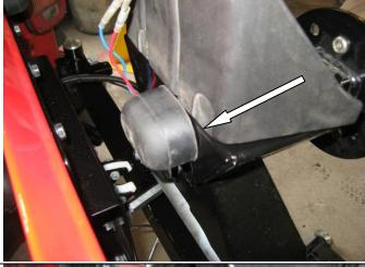
9. **YJ-TJ.** Fit M6 cage nut to inner side of stop light mount and secure rubber stop using original fastener.
