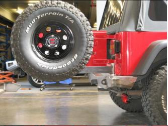
26. Mount spare tyre back to vehicle and check operation of arm. Tighten M20 nyloc on hub to obtain a satisfactory pre-load with door of vehicle. It may be required to slightly adjust the stop assembly for a proper fit.
