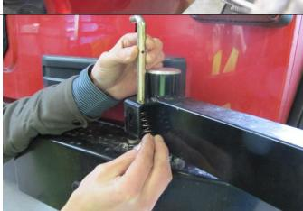
12. **ALL MODELS.** Before fitting arm to vehicle fit lock pin and spring as shown. Make sure the top of the pin faces away from the arm.
