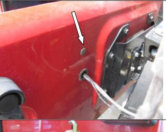
11. Clean area around holes in tailgate.Cover holes in tailgate using the two round self adhesive pads.
