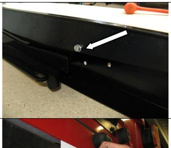
1. Fit cover panel to bar using 4 x m6 x 20 bolts, spring washers, flat washers and flange nuts. Place bolt head towards the outside of the bar.
