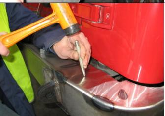
7. If fitting fog light punch out 2 mounting holes in bar as shown.
