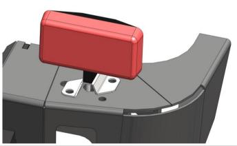
8. Fasten fog light to mount bracket. Secure bracket to bar using 2 x M10 x 35 socket head cap screws, flange nuts.
