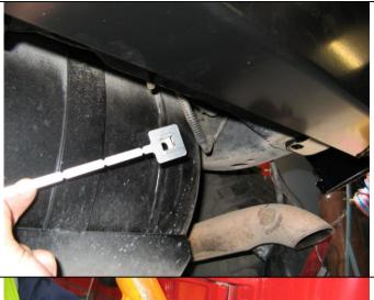
6. Insert M10 cage nuts into cage nut plates. Place cage nut plates on inside of cross member and secure using M10 x 35mm bolts, spring washers and flat washers. Secure outer ends of bar through chassis into end braces using 4 x M10 x 50mm bolts, flat washers, spring washers and M10 nuts. Square bar to vehicle and tighten all bolts.
