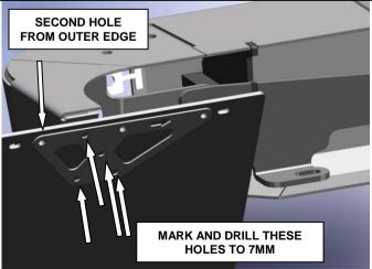
9. If fitting ARB mud flaps use brackets as shown. Arrow in bracket must face towards chassis. Place bracket on mud flap using second hole from outer end. Mark and drill these holes in mud flap to 7mm. Once this is complete fit mud flap to bar using black M6 hardware.
