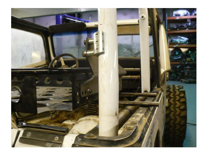
Once both clamps have been bolted to the brackets, attach the outer part of the clamp to both sides of the roll bar. Use the (6)  $5/16 \times 1$ " socket head cap screws and a  $\frac{1}{4}$ " allen wrench. Torque the bolts to 20 ft-lbs in a cross directional pattern.
