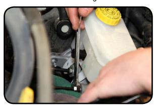
Remove the master cylinder from the vehicle.
