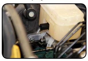
Reinstall the fluid level sensor connector and reservoir cap.
