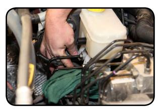
Remove the two mounting nuts that attach the master cylinder to the brake booster using a 13mm deep well socket.
