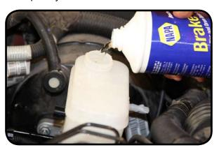
10. Leave the cap off and loosen the brake lines at the master to let the brake fluid bleed through the master. Tighten the brake lines once the reservoir is at operating level. Remove the rags and clean everything with brake cleaner.
