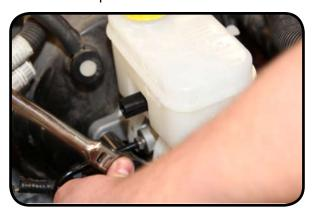
9. Remove the reservoir cap and fill the reservoir completely with DOT 3 brake fluid.
