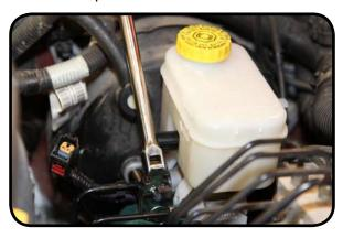
5. Move the master cylinder towards the front of the vehicle roughly 1/2" to release the piston pressure. (If the booster is holding the master in with the vacuum pressure you can remove the check valve at the booster to release the suction from the master.) Remove the brake lines from the master using a 12mm wrench.
