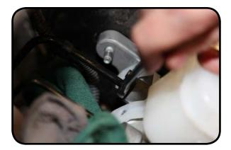
8. After the brake lines are installed into the new master cylinder, install the mounting nuts that secure the master cylinder to the brake booster. Torque to 13 Ft-lbs.
