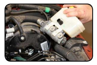
7. Install the new master into the vehicle. Make sure that there is an O-ring seal on the master cylinder where it mounts to the booster. Install the brake lines to the new master.
