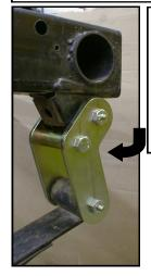
This is the proper way to install the shackles on the FRONT of the YJ. The long leg down, bolt-in center brace back. This way, it acts as a "Anti-Kick-Back" shackle.
