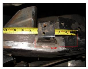
Drivers side: Measure from the Upper Control arm bracket to the back side of the JM700 Mount. This measurement should be **6-1/8**"
