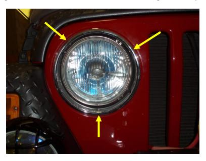
B) There are 2 molded plastic tabs inside the factory bezel that snap it into place. To remove the factory bezel, flex the part toward the inside and pull outward.
