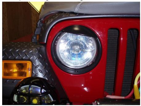
B) Using a #15 torx driver fasten the bezel to the grill with the 3 screws previously removed
