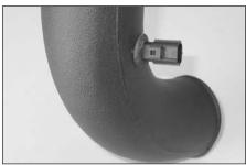
19c. Install the temperature sensor into the grommet as shown.
