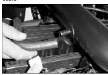
2. Detach the crankcase vent hose from the stock intake tube.
