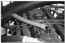
23. Attach the vent hose provided onto the vent fitting on the valve cover and the K&N intake tube.
