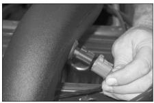
23a. Reconnect the temperature sensor electrical connection.
