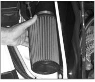
24. Install the K&N Filtercharger element onto the intake tube and tighten the hose clamp provided.
