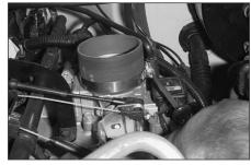
18. Attach the silicone hose to the throttle body using a hose clamp provided.
