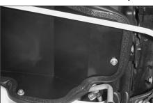
17. Secure the heat shield to the rubber mounted studs using the hardware provided.
