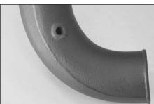
19b. Remove the K&N intake tube from the vehicle and drill a 3/4" hole at the positioned marked in step #19a. Next install the provided grommet into the drilled hole.
