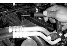
22. Detach the crankcase vent hose from the vent fitting on the valve cover.
