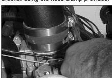
21. Tighten the hose clamp on the silicone hose at the intake tube.
