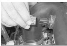
3a. On vehicles equipped with temp sensors, depress the temperature sensor electrical connection locking tab, and then pull on the connector to disconnect the connection.
