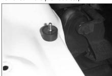
13. Install the second rubber mounted stud into the lower airbox mounting point using the hardware provided.
