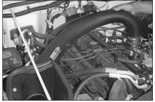
19. Install the K&N intake tube.
