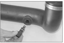
5. On vehicles equipped with temp sensors, lift the temperature sensor-locking tab while twisting the sensor counter clockwise to remove the sensor from the tube.
