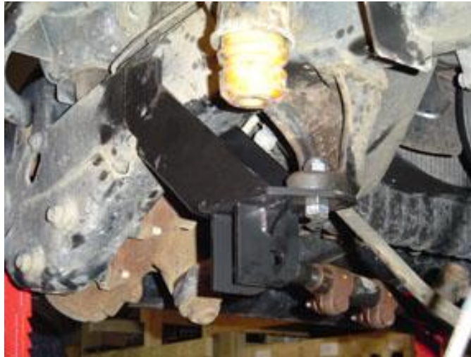
Track Bar Bracket Installed
