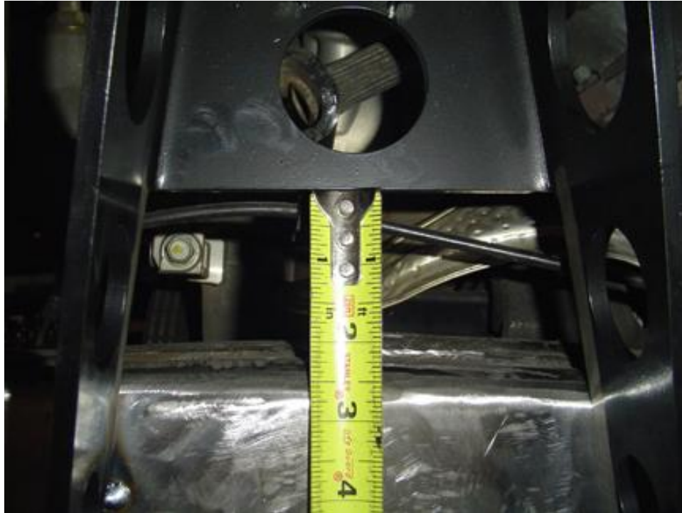
Front Upper Coil Over Mount Positioned on the Frame
