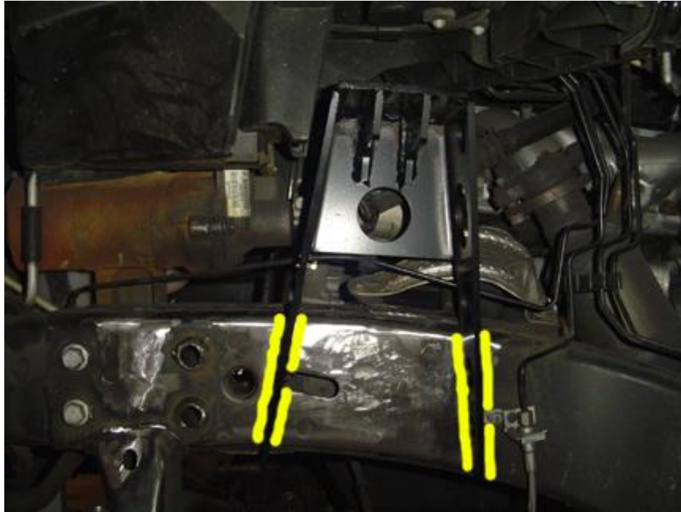
Front Upper Coil Over Shock Mount Welded to the Frame
