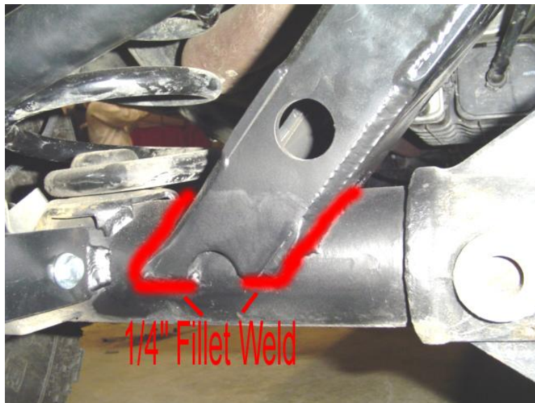
Welding the rear cradle
