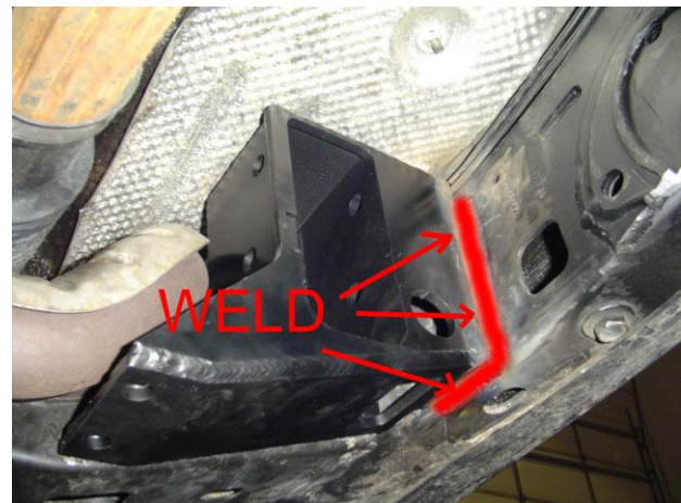
D.S. Bracket Welded in Place
