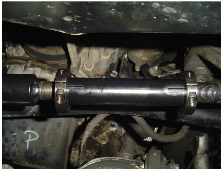
Quick Adjuster with Shaft Collars Installed
