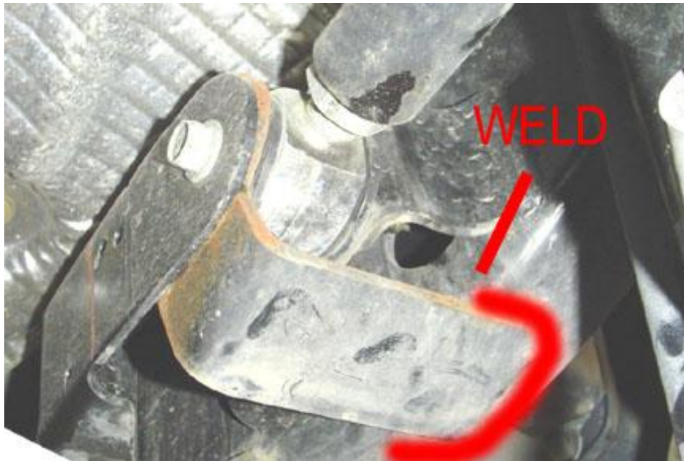
Rear Upper Reinforcing Mounts
