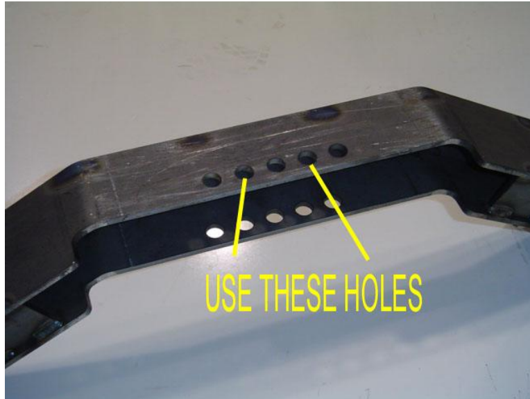
Weld in cradle specified holes
