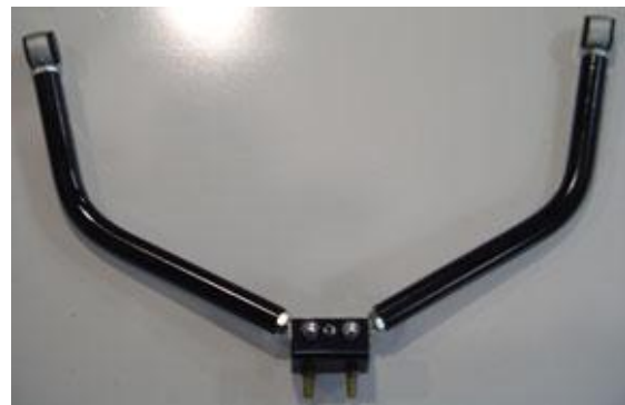
Triangulated 4 -Link Assembly
