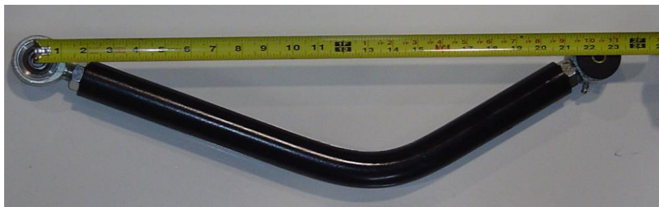
Triangulated 4 -Link Assembly
