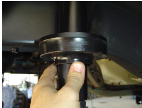
Spring Isolator Installed
