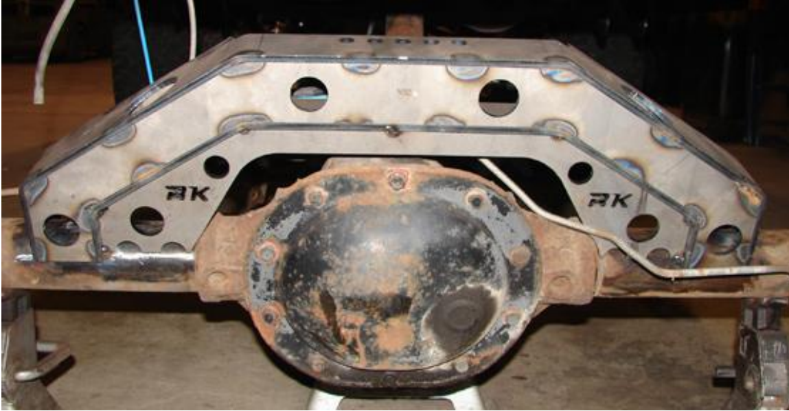
Cradle Tie in Plate Installed
