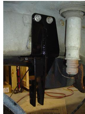
RK Track Bar Bracket Installed
