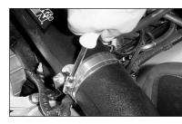
23. Secure the intake tube to the saddle bracket using the hose clamp provided.
