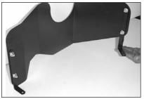
13. Attach the "L" bracket and the twisted "L" bracket to the heat shield using the hardware provided.
