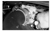
24. Tighten the hose clamp on the silicone hose at the intake tube.
