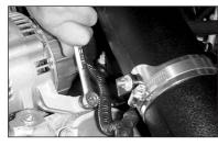
25. Tighten the alternator retaining bolt.
