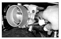
21. Attach the silicone hose to the throttle body using a hose clamp provided.
