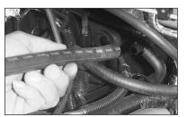
9. Detach the OE crankcase vent hose from the "T" fitting.
