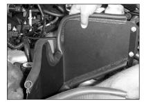
15. Install the heat shield assembly.
