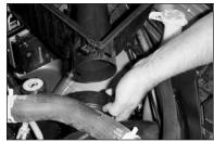
11. Detach the air inlet duct from the airbox base and remove the airbox base.
