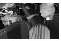
28. Install the K&N Filtercharger element onto the intake tube and tighten hose clamp provided.
