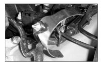
20. Attach the saddle bracket assembly to the alternator using the bolt removed in the previous step. **Note:** Do not tighten completely at this time.
