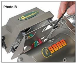
Tighten both 6mm x 1mm x 12 mm screws using a 5mm hex key.
