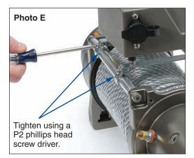
Attach the solenoid pack with mount brackets to tie bars using a phillips head screw with split lock washer.
