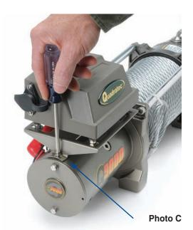
Tighten the third 5mm x 8mm x 12mm screw using a P2 Phillips Screw Driver.
