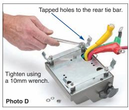
Attach solenoid pack to the top mount brackets using a flat washer, split lock washer and nut for each of the four studs.
