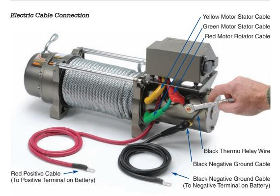
Attach red, yellow and green short cables to motor terminals as shown. Note: The three copper terminal stud ends are color coded. Tighten all three brass nuts onto terminals using a 13mm wrench. **DO NOT OVER TIGHTEN.**
