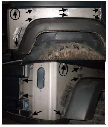
h. Mark both lower LED mounting holes for drilling out to 9/16" once you have removed kit armor panels.
