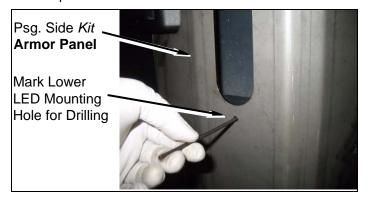
i. Mark three holes surrounging the gas filler hole for drilling out to 1/4" once you have removed *kit* armor panels.
