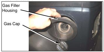
**f.** Reinstall gas cap to prevent any particles from entering the filler tube.
