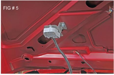
NOTE: If you need to work under the hood for a long period of time, you can turn the hood light off by removing the fuse on the under hood light harness.
