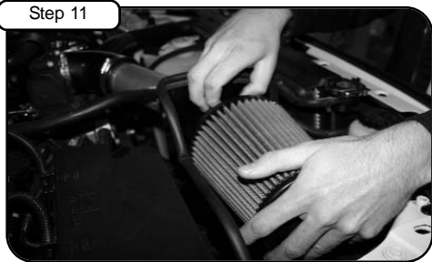
Re-install Crankcase line to new tube with mini clamp #006 provided and tighten using 1/4" nut driver. Place high FLOW filter into housing and tighten using 5/16" nut driver.
