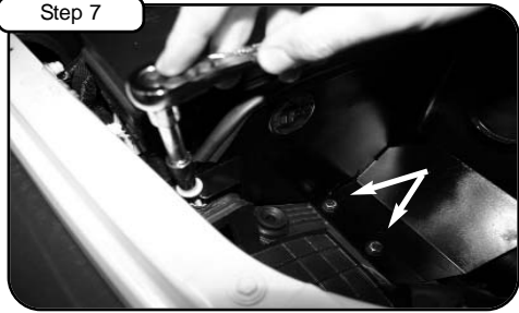
Install trim seal to housing and place in to vehicle. Re-tighten bolt from step 6. With screws provided, tighten down both bolts using 9/16" socket or wrench.
