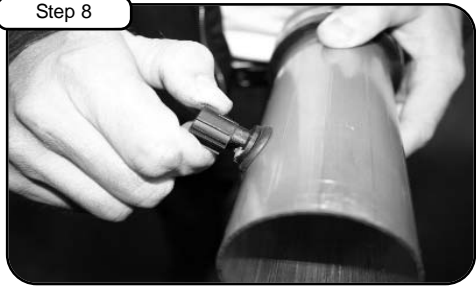
Remove Temp sensor from OE intake tube and place on to new aFe intake tube with grommet provided.
