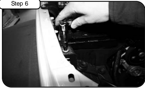
Loosen 10mm bolt holding in airbox bracket.
