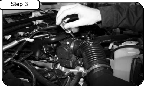
Loosen clamp using 5/16" nut driver @ Throttle body.
