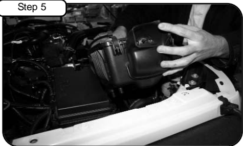
Carefully pull out bottom half of airbox. (caution, this may require some force)
