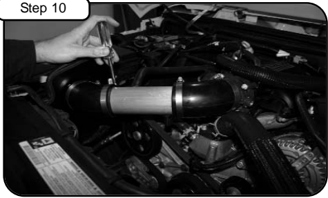
Install 05-00136 end of coupler to housing side and 05-00135 coupler to throttle body side. (make sure temp sensor side of tube is near throttle body side) Tighten clamps using 5/16" nut driver.
