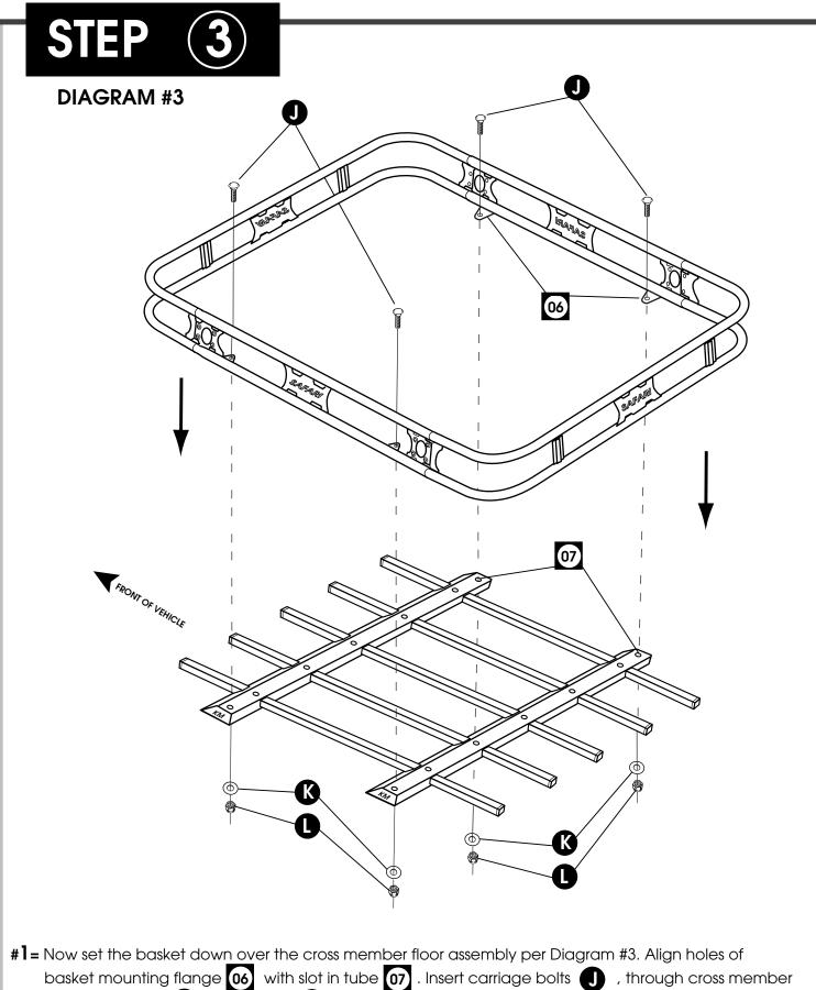
basket mounting flange [06] with slot in tube [07]. Insert carriage bolts [1], through cross member with flat washer (C) and lock nut (1). Center basket on floor assembly and tighten. Now you are ready to install your mounting hardware.
