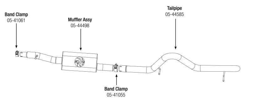
**Step 1:** (Read Instructions prior to installation) Remove your stock exhaust from the rear of your truck working your way forward. Take caution not to damage the factory isolation mounts as they will be reused. It may be helpful to lubricate the isolation mounts prior to disassembly. It is recommended to not fully tighten the clamps until the entire system has been installed.
