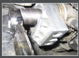
5. Install the oil block off fittings as pictured. Remember, Teflon tape is only to be used on the NPT fittings in the end of the block-off caps. Rubber o-rings should be between the block-off bolt (24mm) and the oil filter block. Torque the 24mm hex head block-off fittings to 25ft/lbs and install the 1/8in NPT pipe thread caps with Teflon tape.
