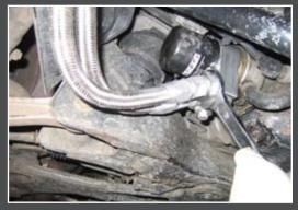
12. Hold the nut that is welded to the cooler core with a wrench and tighten the 90 degree fitting going to the oil cooler core. Failure to hold the nut on the cooler core will damage the core and oil leaks will be a problem. The oil cooler core is made of very thin metal to promote the heat transfer of the oil to air. Do not use any Teflon tape or thread sealer on ANY of the oil cooler line fittings. Serious engine damage and leaks may result from doing so.
