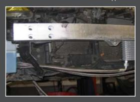
11. Attach the lines to the oil filter block. The oil cooler connections do not have to be installed on any specific port. Use a wrench to hold the fitting oil filter block and to keep it from spinning and tighten the fitting on the oil cooler line. Install the oil filter at this time. The cooler lines should be above the connection for the lower control arm. Lines that are lower than this should be re-located to prevent possible damage from road debris.
