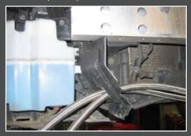
9. Cut another 2-inch x 1.5-inch hole in the inner air diversion plate inside the engine bay directly behind the lower radiator support as shown below. Feed the oil lines around and through both holes to the oil filter block.
