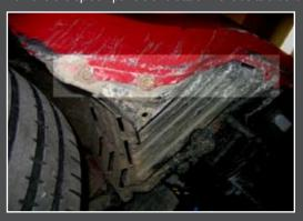
3. Peel the wheel well splash guard out from behind the front bumper near the fenders and remove the (3) 10mm head bolts inside on both sides of the front bumper. (See picture)
