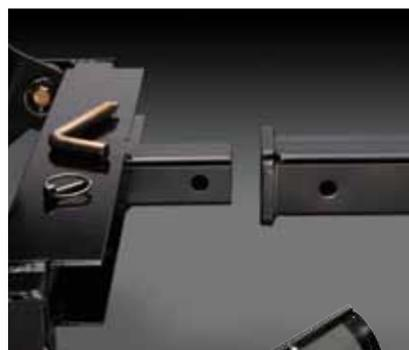
**Quick-Link™:** An easy-to-use mounting system that slides into a Class 3, 2-inch front receiver hitch.\*
