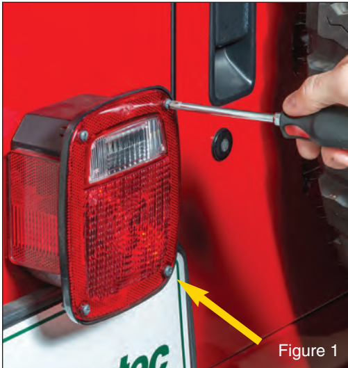
Before you begin installation, put on safety glasses. Start by removing 4 phillips screws.
