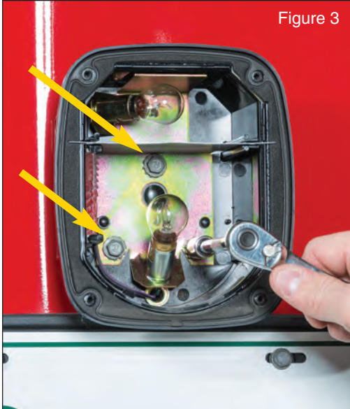
Figure 3: Remove the 3 socket headed screws that attach the taillight to the body of the vehicle using a 3/8" socket.
