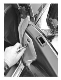
**Step 1**Remove the existing factory mirror using the T40 Torx bit or driver. The two factory fasteners will be re-used to install the new Rampage power mirror system.
