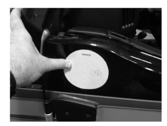
**Step 3**Cut out the template for the door the mirror will be installed on and punch a hole with a pen at the location of the drill point. Align it on the outside of the door as indicated on the pattern. Now mark the drill point on the door.
